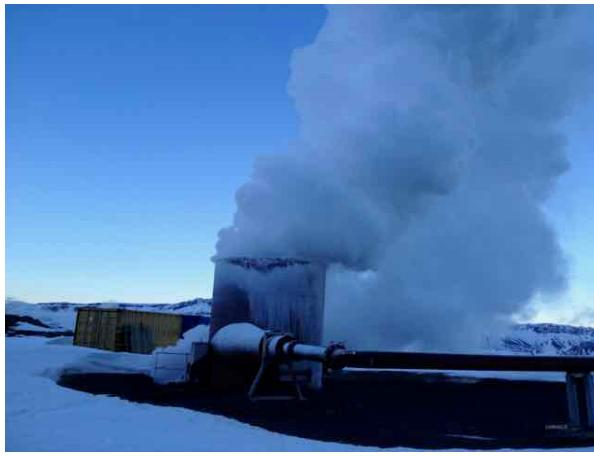
Photo 46: Well test with steam rising through silencer
