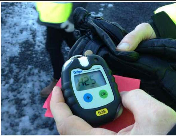
Photo 69: Portable hydrogen sulphide detector
